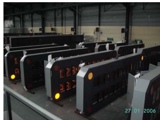
Variable Message Signs (burning test)
