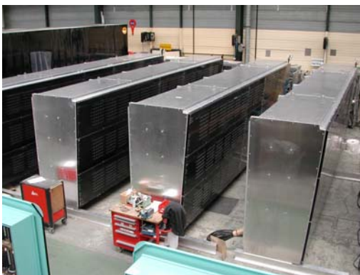
Walk-In VMS in factory
